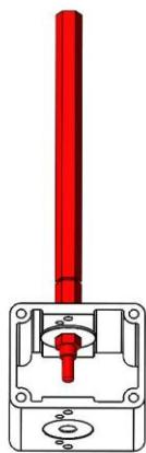
**Step 8:** Place shim washer (am-1444), 20T 0.5in Hex Bore Miter Gear (am-3772), then Output Shaft Spacer (am-1445) onto the output shaft.
